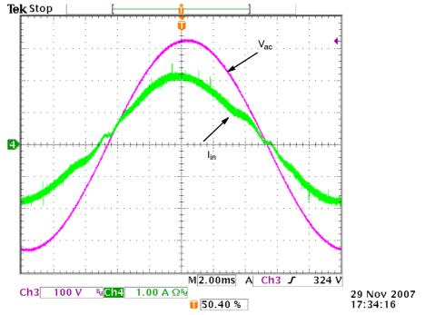
Figure 8. V<sub>ac</sub> = 230 Vac, P<sub>in</sub> = 309 W, V<sub>out</sub> = 393 V, I<sub>out</sub> = 0.77 A, PF = 0.996, THD = 6.1%
