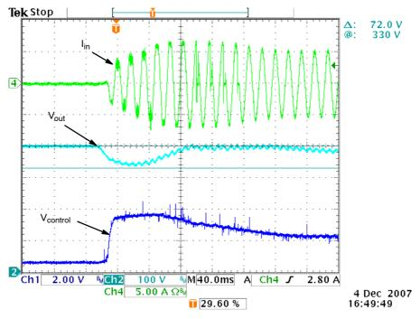
Figure 11. Vac = 85 Vac, Vout = 392.6 V, Iout = 0 A  $\sim$  0.77 A
