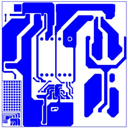
Figure 4. PCB Layout (Solder Side)
