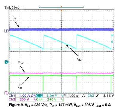
When in light load, the circuit enters a welcome burst mode that enables the circuit to keep regulating.  $V_M$  pin oscillates around its internal reference voltage (2.5 V).
