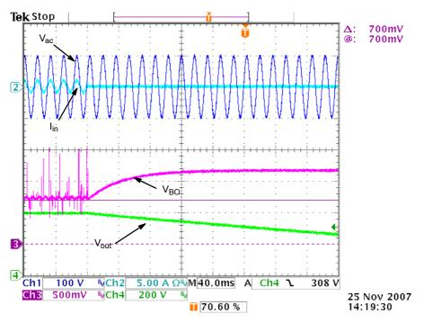
Figure 13.  $V_{ac}$  = 68 Vac,  $V_{out}$  = 393.7 V,  $I_{out}$  = 0.1 A
