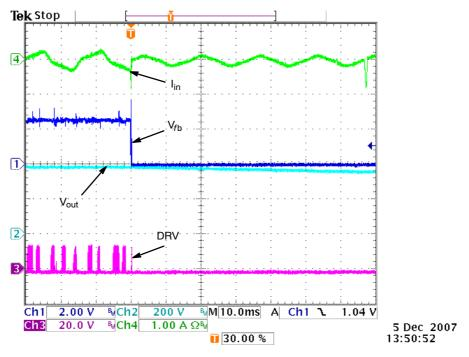
Figure 12. V<sub>ac</sub> = 265 Vac, V<sub>out</sub> = 394.5 V, I<sub>out</sub> = 0.1 A
