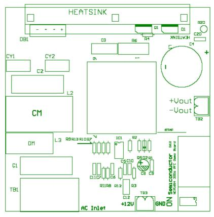
Figure 3. Components Placement (Component Side)
